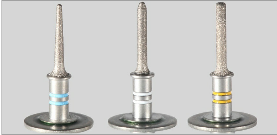
Figure 1.3-1 The three milling burs shown here are used for manufacturing different restorations. The one on the left is used for anterior restorations; the middle for posterior restorations; and the one on the right for the internal intaglio surface of posterior crowns.
